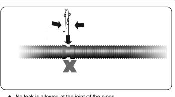
No leak is allowed at the joint of the pipes
